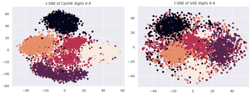
Figure 3: Visualization of subgroups within MNIST digit population after t-SNE projection of latent space for our method (left) vs a standard VAE (right). Each color represents one of the five digits within the population.
