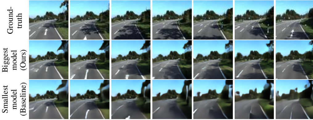
Figure 6: KITTI driving qualitative evaluation. Our highest capacity model (middle) is able to maintain the observed dynamics of driving forward and is able to generate unseen street lines and the moving background. The baseline (bottom) loses the street lines and the background becomes blurry. For best viewing and more results, please visit our website https://cutt.ly/QGuCex .
