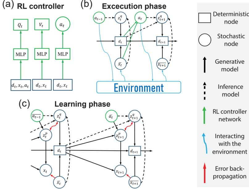
Figure 2: Computation graph of the proposed algorithm. **(a)** The RL controller. **(b)** The execution phase. **(c)** The learning phase of a VRM.  $a$ : action;  $z$ : latent variable;  $d$ : RNN state variable;  $x$ : raw observation (including reward);  $Q$ : state-action value function;  $V$ : state value function. A bar on a variable means that it is the actual value from the replay buffer or the environment. Each stochastic variable follows a parameterized diagonal Gaussian distribution.
