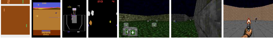
Figure 3: Screen shots of Atari games and ViZDoom tasks. From left to right, they are Pong, ChopperCommand, DoubleDunk, Asteroids, Health Gather, Health Gather v2 and Defend Center. When only given one frame as the input, these Atari games are POMDPs because we can not obtain the velocity of the moving object from a single observation. Because the agent in ViZDoom environment can only see in just one direction, it naturally introduces partial observability to these tasks.
