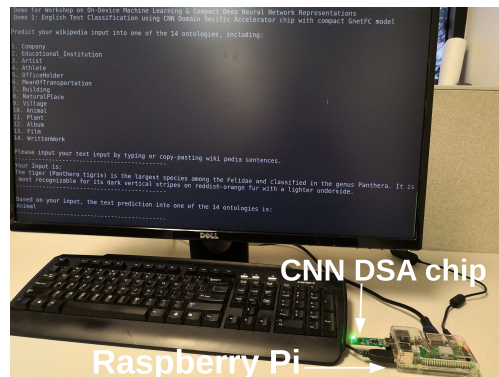
Figure 1. Efficient On-Device Natural Language Processing system demonstration. The CNN-DSA chip is connected to Raspberry Pi through the USB interface. Keyboard sends the typing text input to Raspberry Pi through USB. A monitor is connected to Raspberry Pi through HDMI for display. On the monitor, it shows the introduction for the demo (zoom in to see details). There are two demos. The first demo classifies the input English Wikipedia sentence into one of the 14 ontologies. The second demo classifies the Chinese online-shopping review into positive or negative.
