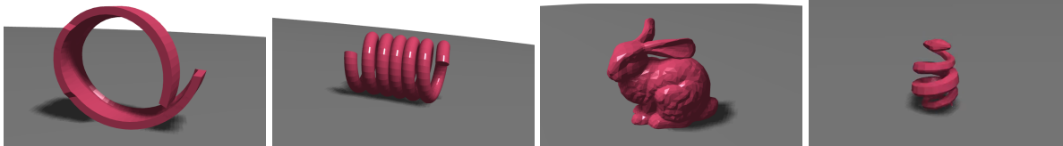
Figure 1: Examples from our supplementary video, showing self collision for the bracelet, spring, bunny, and snake models. Self-collision is identified using a learned neural network SDF, and collision response uses the SDF gradient computed via back-propagation within a constraint solver. Neural SDFs work well for low dimension reduced spaces (e.g., the bracelet and spring with dimension 3), while models that need more dimensions to provide good reduced deformation models (e.g., the bunny with dimension 10, and the snake with dimension 7) have much less accurate learned collision manifolds.
