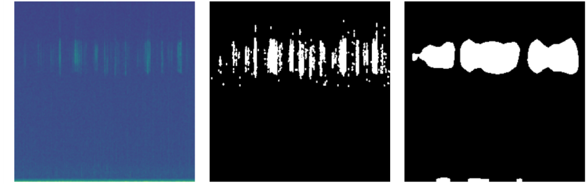
Figure 3: Spectrogram ( left ), high-quality segmentation mask ( middle ), and generated pseudo-attention mask ( right ) for a recording of porpoise clicks.
