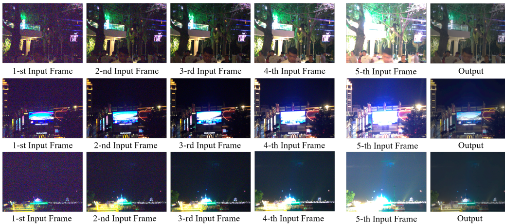
Figure H: Full-image results on the real-world dataset of BracketIRE+ task. Our results preserve both the bright areas in short-exposure images and the dark areas in long-exposure images. Note that the size of the original full images is very large, and here we downsample them for display. Please zoom in for better observation. Moreover, we provide a higher resolution version in README.md of the supplementary material.
