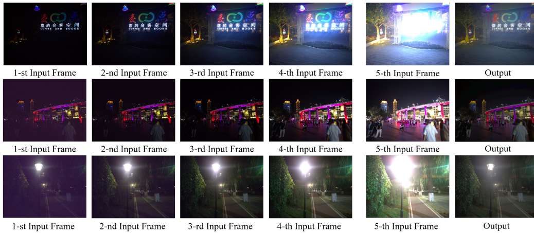
Figure G: Full-image results on the real-world dataset of BracketIRE task. Our results preserve both the bright areas in short-exposure images and the dark areas in long-exposure images. Note that the size of the original full images is very large, and here we downsample them for display. Please zoom in for better observation. Moreover, we provide a higher resolution version in README.md of the supplementary material.
