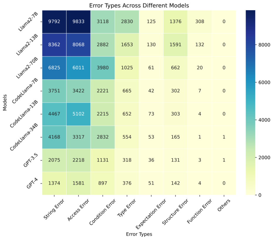
Figure 5: Distribution of error types among different LLMs on WikiSQL. Definitions of error types and prompts for error classification are put in Appendix.
