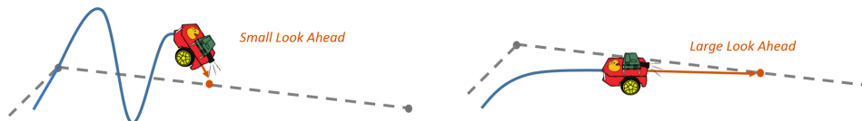
Figure 2: The operation of the pure pursuit controller.
