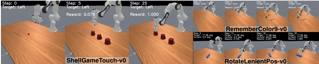
Figure 2: Illustration of demonstrative memory-intensive tasks execution from the proposed ManiSkill-Memory benchmark. The ShellGameTouch-v0 task requires the agent to memorize the ball’s location under mugs and touch the correct one. In RememberColor9-v0 , the agent must memorize a cube’s color and later select the matching one. In RotateLenientPos-v0 , the agent must rotate a peg while keeping track of its previous rotations.
