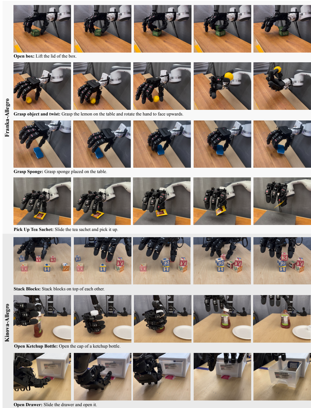
Figure 7: Real world task rollouts demonstrating the ability of OPEN TEACH to perform intricate, long-horizon tasks.
