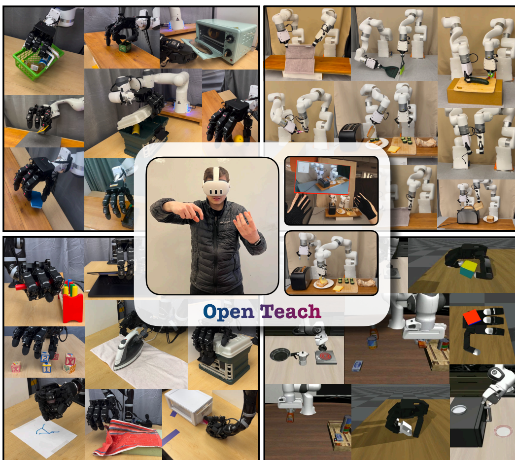
Figure 1: We present OPEN TEACH, a unified robot teleoperation framework that supports multiple arms and hands, allows mobile manipulation, is calibration-free, and works across both simulation and real-world environments. OPEN TEACH uses a VR headset for teleoperation, offers low latency and high-frequency visual feedback. This high-frequency operation allows human users to correct for robot errors in real time, facilitating the execution of intricate and long-horizon tasks. From making a sandwich and ironing cloth to placing items in a basket and lifting it and approaching a cabinet and opening it , OPEN TEACH delivers a comprehensive, user-friendly teleoperation experience for a wide range of applications. OPEN TEACH is fully open-source.
