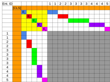
Figure 2: Example attention mask for our approach. Ent. ID included for illustration purposes only. E2E attention denoted in yellow.
