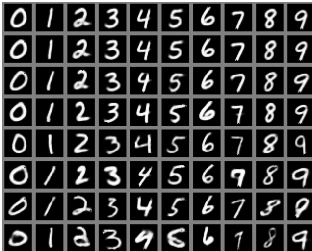
Figure 1: Generated digits images. From left to right, we have the ten classes found by DAC and ordered thanks to the Hungarian Algorithm. From top to bottom, we go further and further in random directions from the centroids (the first row being the decoded centroids).
