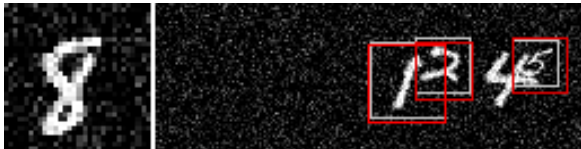
Figure 4: A query digit (left) and a set of digits (right) for the proposed CAPTCHA test. The ground truth and our predicted solutions are shown by white and red boxes respectively.
