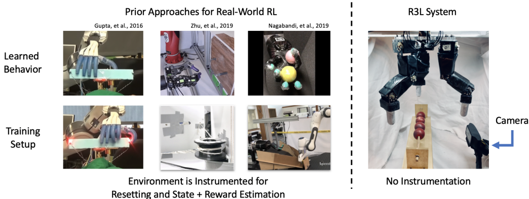
Figure 2: We draw a comparison between current real world learning systems which rely on instrumentation versus a system that learns in an environment more representative of the real world, free of instrumentation. While all three prior works utilize instrumentation for resets, state estimation, and reward, the motion capture system of Gupta et al. (2016), sensor attached to the door in Zhu et al. (2019), and auxiliary robot which picks up fallen balls in Nagabandi et al. (2019) are good examples of engineered state estimation, reward estimation, and reset mechanisms respectively.
