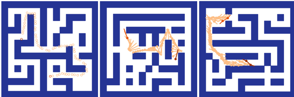
Figure 15: The solution path produced by NEXT in a workspace planning task (2d), rigid body navigation task (3d), 3-link snake task (5d) from left to right. The orange dot and the brown dot are starting and goal locations, respectively.
