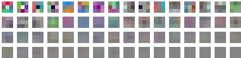
Figure 5: Visualization of filters in the first convolutional layer of VGG-16 trained on CIFAR-10. Filters are ranked by \ell_1 -norm.
