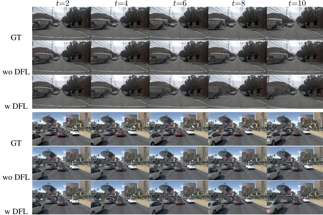
Figure 5: Visualization. Comparison of future frame predictions with and without Dynamic Focal Loss (DFL). The first row shows ground truth frames, the second row shows predictions without DFL, and the third row shows predictions with DFL. Sampled frames at t=2, 4, 6, 8, 10 are shown.
