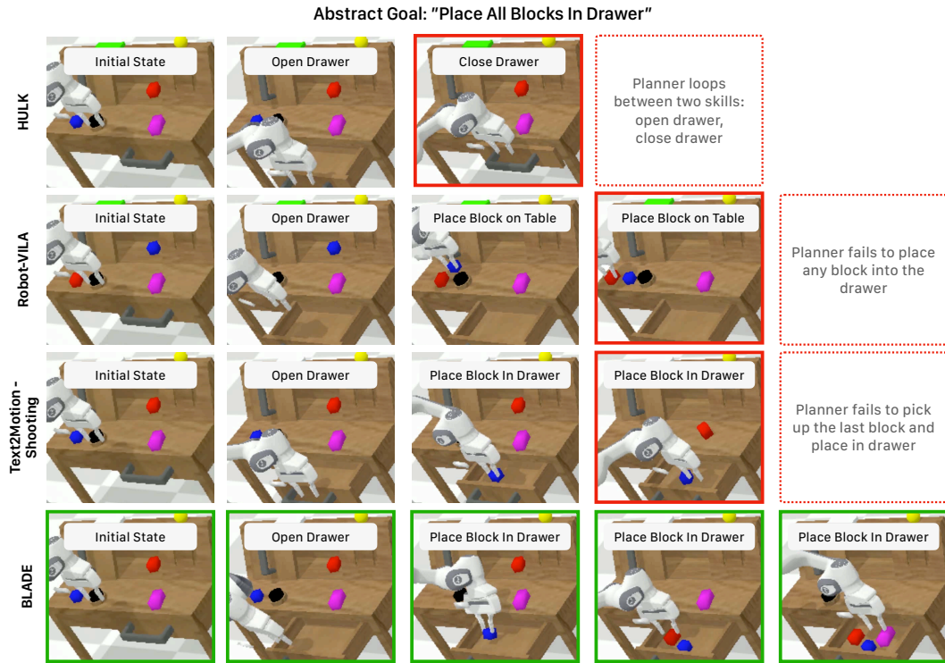
Figure A2: BLADE and baseline performance on an Abstract Goal generalization task in the CALVIN environment.
