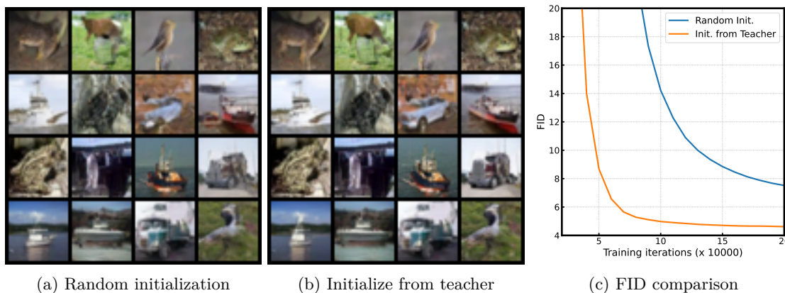
Figure 4: Comparison between student model weights random initialized and initialized with teacher model weights on CIFAR-10 dataset.
