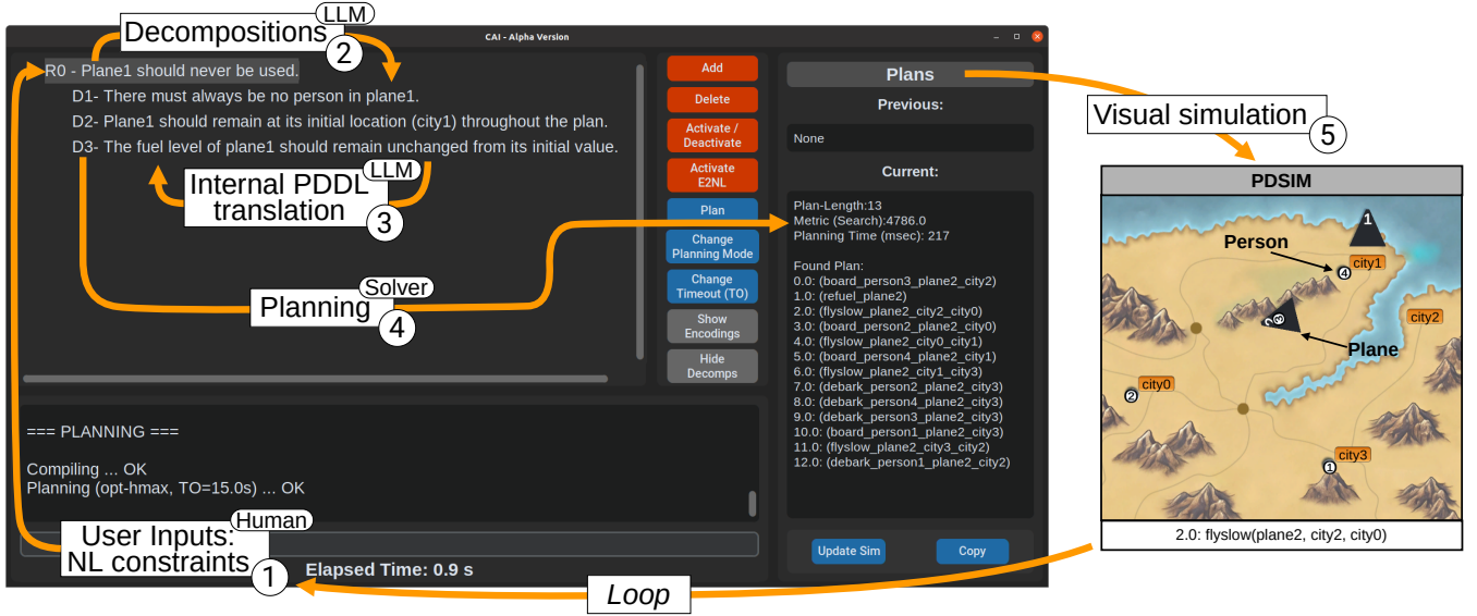
Figure 2: Main interface and workflow. ① The user provides a natural language constraint. ②-③ The input is translated using our proposed interactive translation pipeline. ④ The problem is solved with the active constraints. ⑤ The generated plan is simulated in PDSim. Based on visual feedback, the human can iteratively refine the solution by adjusting the constraints.
