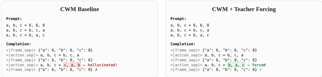
Figure 4: Illustration of action hallucination and teacher forcing in a CWM trace. Left: In the baseline setting, an incorrect next command corrupts the execution history and forces all subsequent states to be wrong. Right: Under teacher forcing, the ground-truth command is injected at each step and evaluation isolates state prediction.
