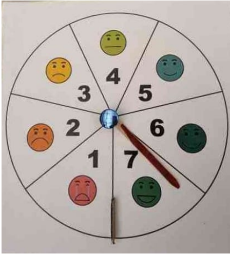
Figure 3: Seven-position rotary knob to elicit comfort ratings
