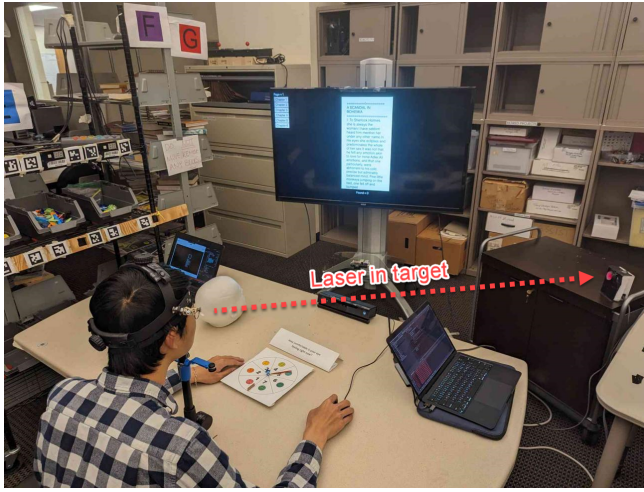
(a) Text is displayed when the laser is pointed to the photo-resistor apparatus
