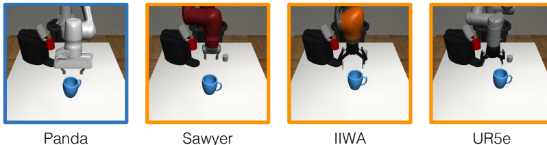
Figure E.1: Robots used in Robot Transfer Experiment. The figure shows the robot arms used for data generation. Source datasets were collected on the Panda arm (blue border) and used to generate data for the Sawyer, IIWA, and UR5e arms (orange border).
