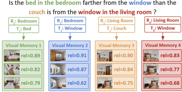
Figure 4. FAST-EQA employs a bounded memory system that allocates a dedicated visual memory for each target, retaining the k most relevant images (here, k = 3 ). The overall memory footprint scales only with the number of targets and remains constant over time, even in long-horizon tasks.
