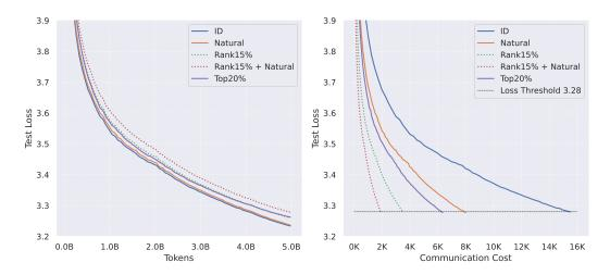
Figure 6: Left: Test loss vs. # of tokens processed. Right: # of bytes sent from each worker to the server normalized by model size to reach test loss 3.28. Rank/TopX% = Rank/TopK compressor with sparsification level X%; ID = no compression.
