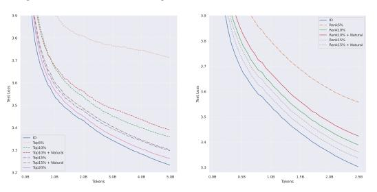
Figure 7: Test loss vs. # of tokens processed. Top/RankX% = Top/RankK compressor with sparsification level X%; ID = no compression. "+ Natural" corresponds to applying Natural compression after Top/RankK compressor. Experiments use a tokens budget of 2.5B.
