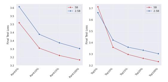
Figure 5: **Final test loss vs. compression parameter** K**.** Results are shown after processing 5B tokens (red) and 2.5B tokens (blue) for RankK (left) and TopK (right) compressors. K=100% corresponds to the non-compressed baseline. In the TopK plot, the 2.5B setup outperforms 5B due to differences in scheduler behavior, as the runs execute a different number of steps.
