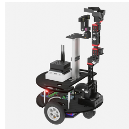
Fig. 4. Blender render of the “Armstrong” rover. This model is based on the CAD design for the rover and conserves the collision model. Each component was textured to increase the visual fidelity of the model.
