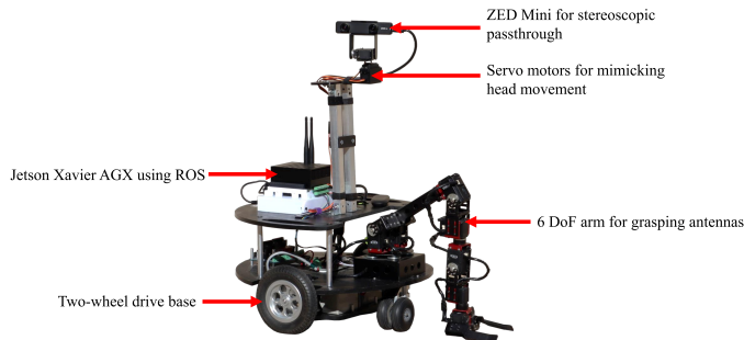
Fig. 2. The “Armstrong” rover. Its robotic arm allows for it to manipulate items such as antenna nodes in its environment. It is also equipped with a ZED Mini to give the operator a first-person perspective from the rover.
