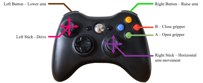
Fig. 3. “Armstrong’s” Xbox 360 button mapping. This popular gamepad makes “Armstrong’s” control feel more intuitive to the operator.
