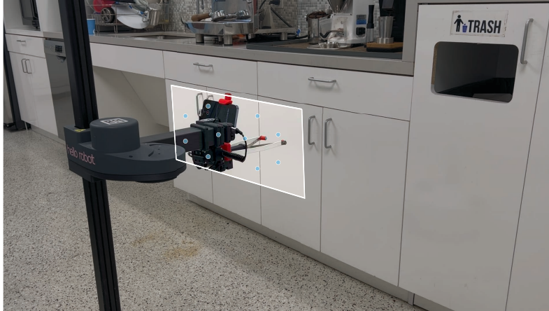
Figure 12: 10-run evaluation schedule used to evaluate Robot Utility Models, with robot starting positions denoted by the pale blue dots in the image. We assume that the robot is at the task space facing the object, but it can be at different offsets with respect to the target object. On our object centric tasks (reorientation, bag and tissue pickup) we also randomize the position of the object itself.
