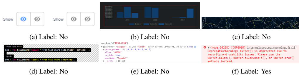
Figure 10: Examples of images that cannot (top row) and can (bottom row) be processed into text by OCR software. Typically, code and webpages are OCR-able while diagrams, plots, and art are not.
