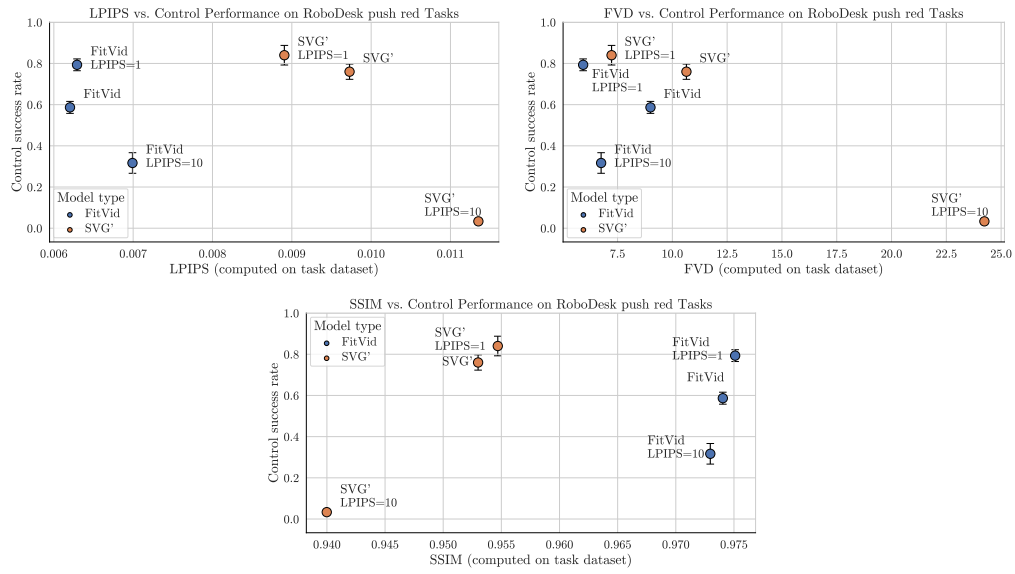
Figure 8: Detailed results comparing perceptual metric values and control performance: RoboDesk push red button task.
