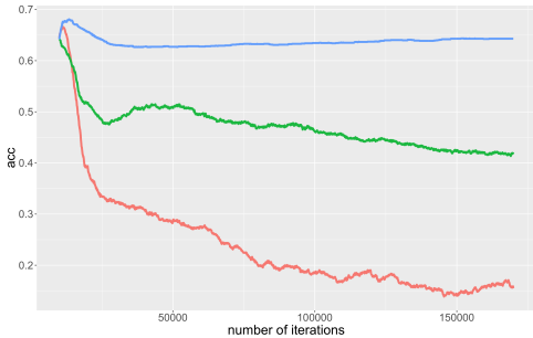
Figure 1: Accuracy of GCN by attacking features, edges or both, with Cora dataset. Green: attacking edges; blue: attacking features; red: attacking both.
