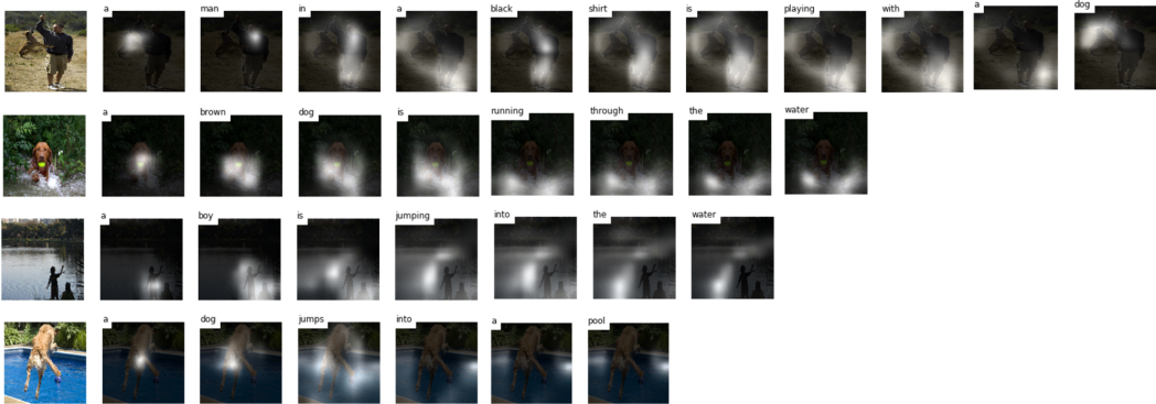
Figure 4: Results on training an image captioning model with visual attention mechanism (Xu et al., 2015) on the Flickr8k dataset using experimental technique (PB). The predicted word and attention weights for each timestep are shown for 4 generated captions of different lengths
