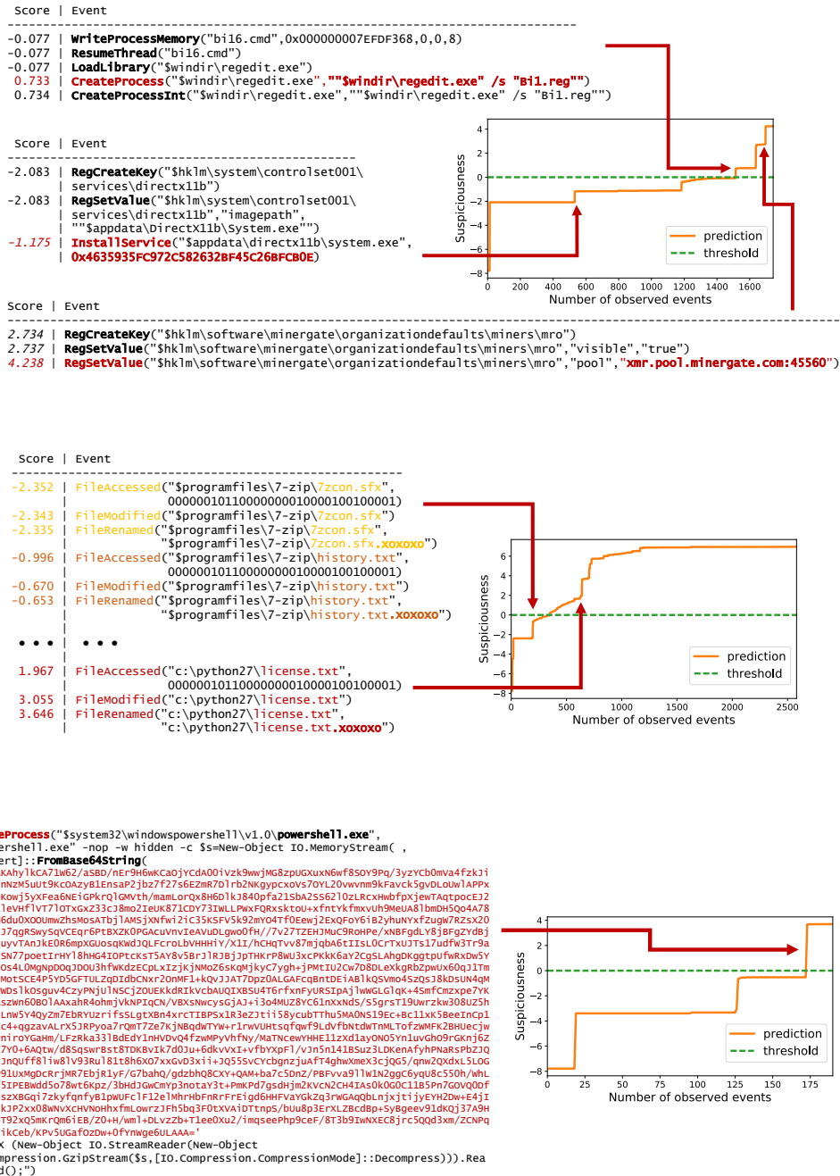
Figure 2: Predictions of the deep monotonic model for three malicious logs alongside with the suspicious lines from these logs.
