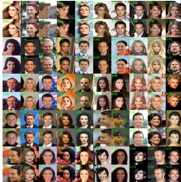
Figure 14: Benign samples (on odd rows) and adversarial samples of standard discriminator (on even rows). Confidence is depicted at corner. Standard discriminator is extremely vulnerable to imperceptible perturbation. The perturbation level is 1/255 .
