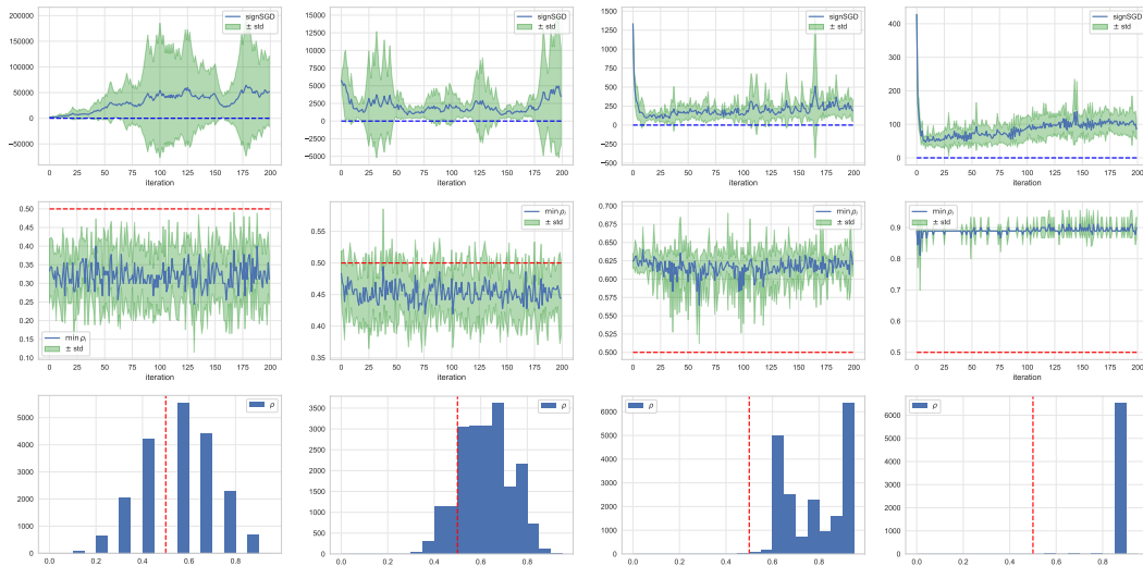
Figure 4: Performance of signSGD with constant step size ( \gamma = 0.25 ) under four different noise levels (mini-batch size 1, 2, 5, 8) using Rosenbrock function. Each column represent a separate experiment with function values, evolution of minimum success probabilities and the histogram of success probabilities throughout the iteration process. Dashed blue line in the first row is the minimum value. Dashed red lines in second and third rows are thresholds 1/2 of success probabilities. The shaded area in first and second rows shows standard deviation obtained from ten repetitions.
