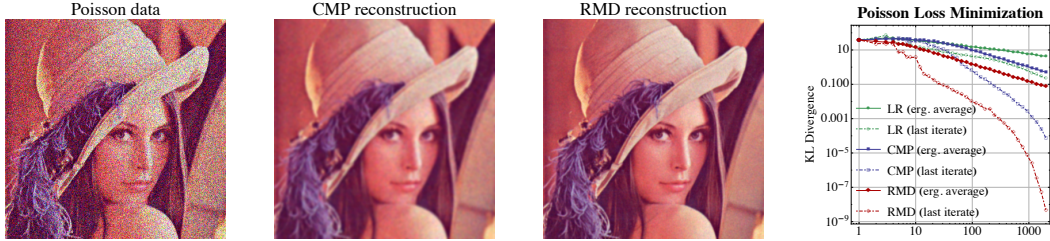
Figure 1: Reconstruction of the Lena test image from a sample contaminated with Poisson noise. Left to right: (a) the contaminated sample; (b) CMP reconstruction; (c) RMD reconstruction; and (d) Poisson likelihood loss at each iteration. The RMD process provides a sharper definition of image features relative to the CMP algorithm (which is the second-best).
