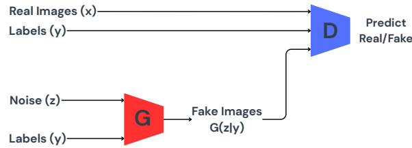
Figure 3: Architecture of a Conditional GAN (cGAN). The generator and discriminator are both conditioned on auxiliary information, such as class labels, allowing the model to generate data that adheres to specific conditions.
