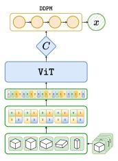
Figure 5: sViT architecture. The input is a set X of images. These are split in non-overlapping patches and fed to a transformer encoder using a shared positional encoding, as indicated by the patch colors. The sViT outputs a context as a vector (V) or collection of visual tokens (T). The DDPM is conditioned on this information using FiLM or attention.
