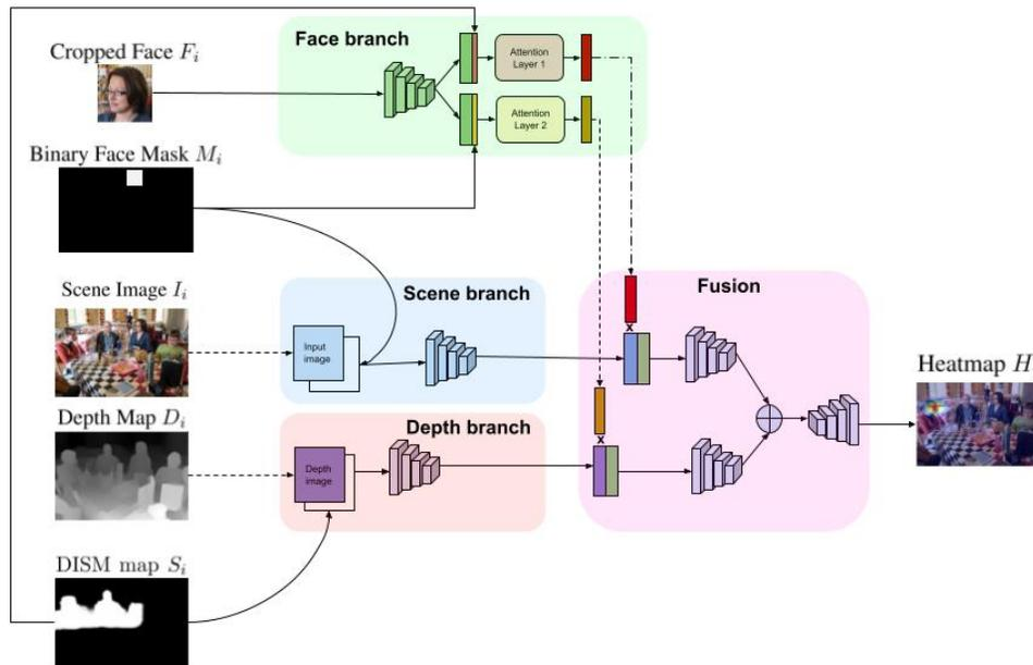
Figure 3: Our MMF module comprises three branches - face, scene, and depth. The three branches are fused in the Fusion module. The output of the module is a 2D Heatmap  $H_i$  superimposed on the scene image  $I_i$  here for visualization.
