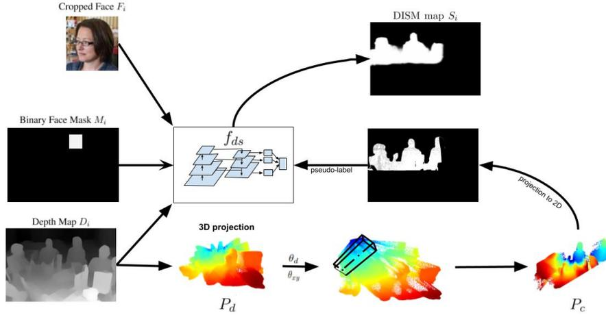
Figure 2: Overview of DISM. We take 3D projection of depth map  $P_d$  alongside gaze binning parameters  $\theta_d$  and  $\theta_{xy}$  to extract a sub-collection of filtered 3D points  $P_c$ . The re-projection of  $P_c$  back to the image-plane serves as pseudo-labels for the FPN network,  $f_{ds}$ . The network provides a representation of the learned DISM map  $S_i$ .
