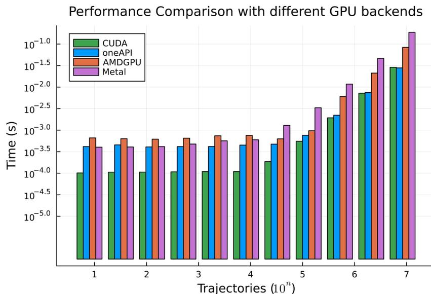
Figure 10: A comparison of the time for an ODE solve for adaptive time-stepping, measured on different GPU platforms. The stiff ODE solver `GPUrosenbrock23` is used here. We measure the time (*lower the better*) versus the number of parallel solves. Here, the NVIDIA GPUs perform the best owing to the most-optimized library and matured ecosystem with JuliaGPU.
