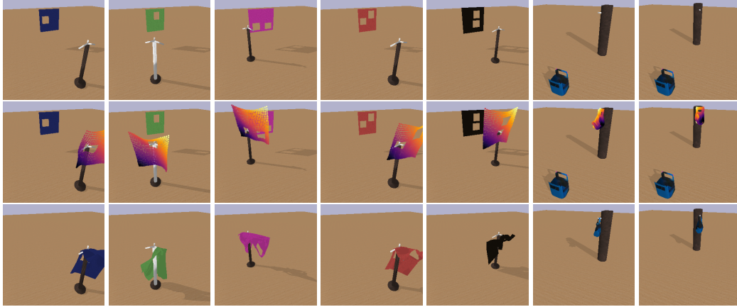
Figure 3: TAX3D generalizes to diverse cloths and anchor positions ( top ); we also visualize the corresponding goal predictions ( middle ) and successful rollouts ( bottom ) after releasing the cloth. The two rightmost columns are HangBag configurations - all others are HangProcCloth configurations.
