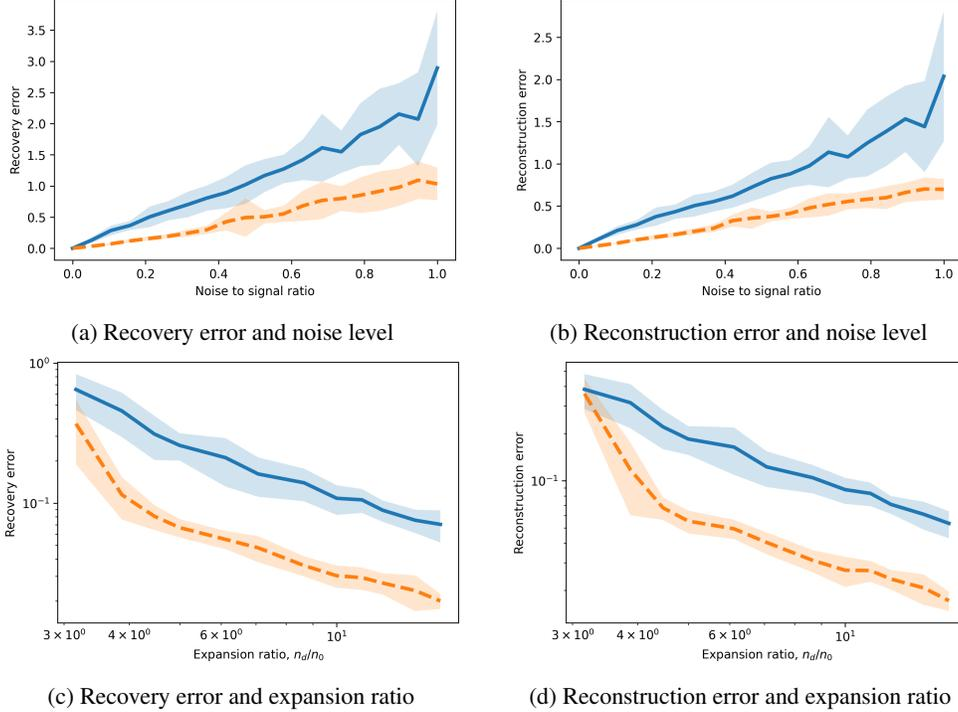
Figure 2: Comparison of PLUGIn (solid line) with gradient descent (dashed line). Panel (a) shows the dependence of relative recovery error with noise level-to-signal level from 20 independent trials. Panel (b) shows the dependence of relative reconstruction error and noise level-to-signal level. Panel (c) and (d) shows the dependence of relative recovery error and reconstruction error, respectively, with respect to the expansion ratio  $n_3/n_0$ .
