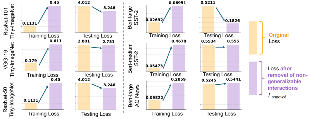
Figure 4: The change of the cross-entropy loss when we remove non-generalizable interactions from the network output v_{\text{removed}}(\mathbf{x}) . The removal of non-generalizable interactions significantly increases the training loss, which restores the training loss that was inappropriately depressed by overfitted representations. In comparison, the testing loss either decreases significantly or does not change a lot.
