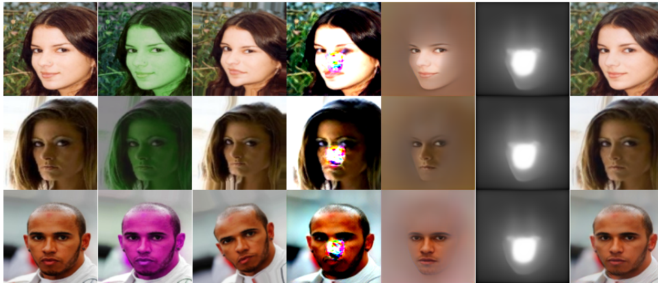
Figure 6: From left to right input image, color jittered image, thin-plate-spline warped image, reconstructed background, predicted foreground, mask, and reconstructed output.
