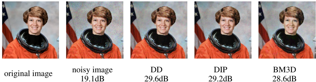
Figure 2: An application of the deep decoder for denoising the astronaut test image. The deep decoder has performance on-par with state of the art untrained denoising methods, such as the DIP method (Ulyanov et al., 2018) and the BM3D algorithm (Dabov et al., 2007).
