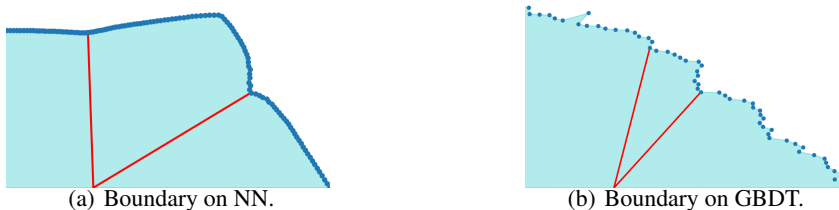
Figure 1: Decision boundary (NN and GBDT models on MNIST dataset) projected on a two-dimensional hyperplane. To choose which 2D hyperplane to project to, we run a decision-based attack from two random initialization points, and use their converged perturbation directions as the vector to form the hyperplane. We then query the decision boundary on this hyperplane to plot these figures.
