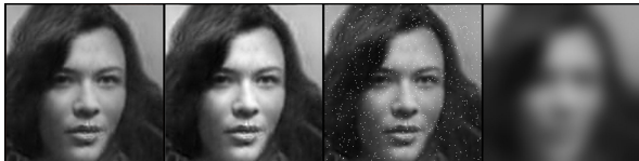
Figure 1: From left to right, the images are the original image, a contrast stretched image, an image with impulsive noise contamination, and a Gaussian smoothed image. Although these images differ greatly in quality, they all have the same MSE from the original image (about 400), suggesting that MSE is a limited technique for measuring image quality.
