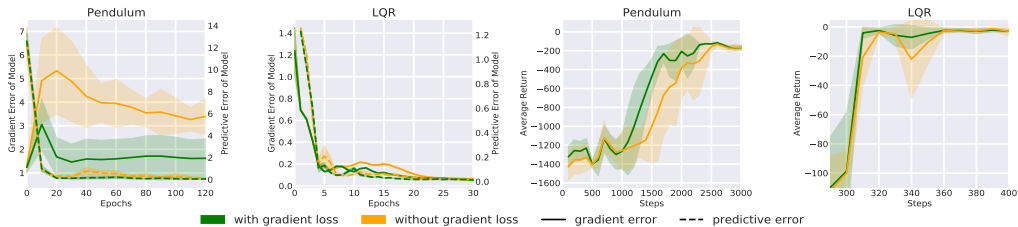
Figure 2: The left two figures show learning curves of models with and without gradient loss on two simple environments. Data used to train each model is collected by a random policy. Solid curves express the mean of gradient error of five trials. Dotted lines express the mean of prediction error during the training of the model. Shaded regions correspond to standard deviation among five trials. The model with gradient loss has a lower gradient error than the model without gradient loss. The improvement is more pronounced in nonlinear cases, i.e., Pendulum environment. The right two figures show the overall performance of using two different types of model, which yields the importance of considering the gradient loss.
