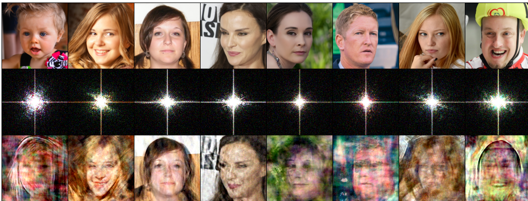
Figure 13: Qualitative visualization of using greedy guidance to solve the Phase retrieval inverse problem. Top row is the ground truth, middle row is the measurement, and the bottom row is the reconstruction.
